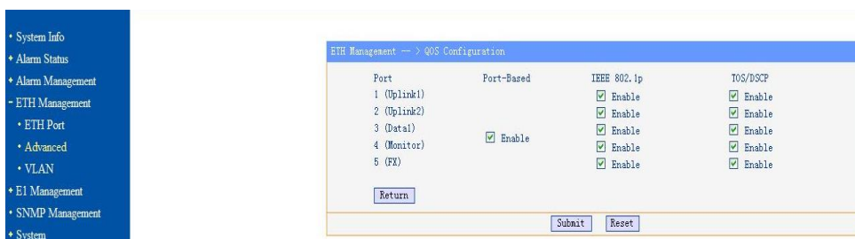
Fig 5.4-3 Ethernet QoS configuration
